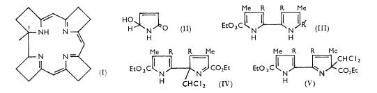
an NH band of approximately one half the intensity of the original as well as two nonequivalent esters. Analysis indicated that the elements of dichlorocarbene had been added to the original bipyrrole, and the nuclear magnetic resonance spectrum of the product showed the presence of a new proton  $(\tau, 3.42)$  together with the absence of aliphatic methyl groups. All of this evidence was consistent with the structures (IV) or (V) for the irradiation product.
