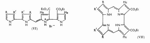
without isolation, with diethyl 4,4'-dimethyl-2,2'-bipyrrole-3,3'-dicarboxylate in presence of hydrobromic acid, and the purple product identified as (VI; R = R' = Me), a member of the 5,5'-di(pyrrol-2-yl)dipyrromethenes. Such compounds have been prepared previously<sup>9</sup> by condensation of 5-formyl-2,2'-bipyrroles with unsubstituted 2,2'-bipyrroles.
